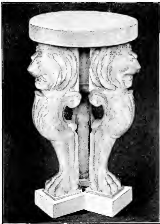
Fig. 69 --Concrete Table, the Legs of which were Cast in a Glue Mold
